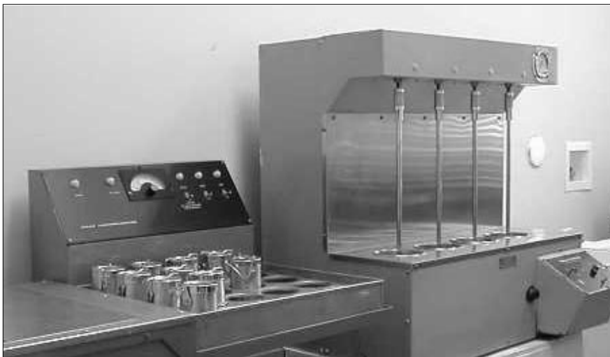
Figure 1: Terg-o-tometer for evaluating laundry products on a laboratory scale
